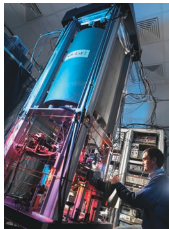
The caesium fountain atomic clock NPL-CsF2 in the National Physics Laboratory in the UK.
